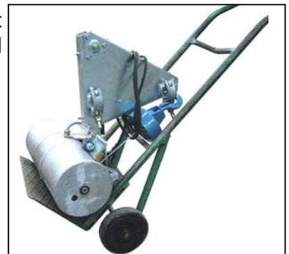
Fig. 9 Transporting the winch
